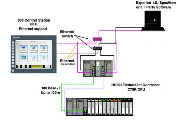
Connect to C70R using dual Ethernet cables.
