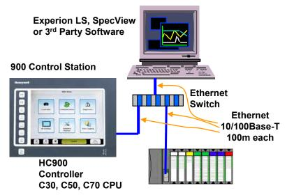
Use shielded CAT5 cable with RJ45 connectors. Connect to HC900 Ethernet port. (On models C70 and C70R with two ports E1 and E2; either port can be used.)
