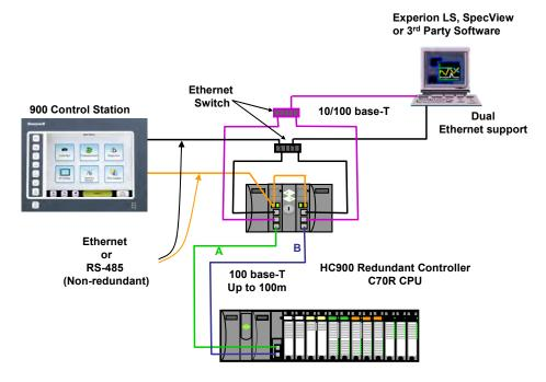
Connect to C70R using either RS-485 or Ethernet. Communication redundancy is not supported using both RS 485 and Ethernet. Communications to the Lead CPU is maintained following a CPU failover event.
