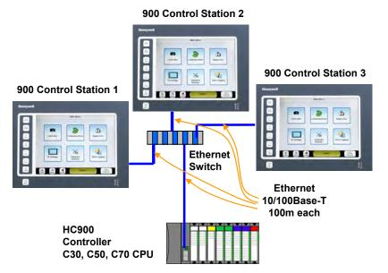
Up to 3 Control Stations may be connected to a HC900 controller using Ethernet. Multiple stations via RS 485 are not supported.
