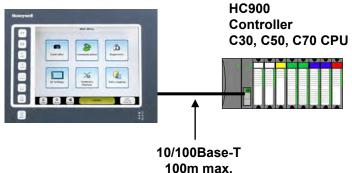
Use shielded CAT5 cable with RJ45 connectors. Connect to HC900 Ethernet port. (On models C70 and C70R with two ports E1 and E2; either port can be used.)
