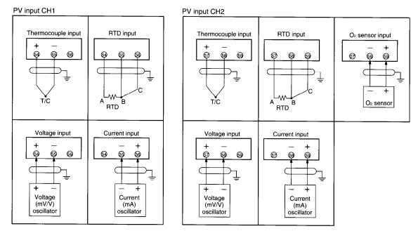
Note: If voltage mode signals are input to PV input CH1 (terminal Nos. (5), (6)) and input CH2 (terminal Nos. (3), (9)) for current input by mistake, a large current might flow and cause the controller to malfunction. Before wiring to the current input terminals on the **DCP552**, make sure that current input signals are output correctly within the range 4 to 20 mA.
