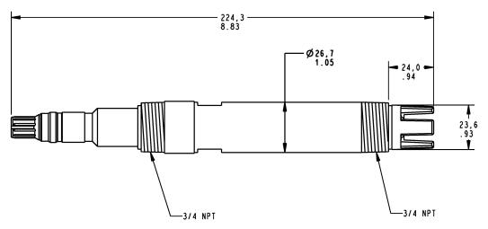
Durafet III (Vario Pin Connector) pH Electrode for Immersion Mountings (Guarded Tip)
