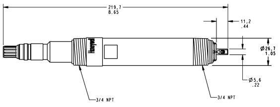
Durafet III (Vario Pin Connector) pH Electrode for In-Line Mountings (Smooth Tip)
