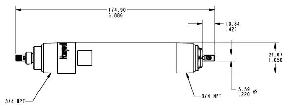
Durafet II (PC Board Connector) pH Electrode for In-Line Mountings (Smooth Tip)
